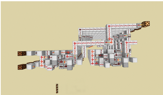
Fig. 16. Two's complement subtraction unit in Minecraft 1.18.2. The SUB control signal feeds into XOR gates on the B input line and sets Cin = 1 on the least significant adder stage, enabling subtraction via two's complement negation.
